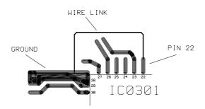
Location of wire link on component side of PWB
